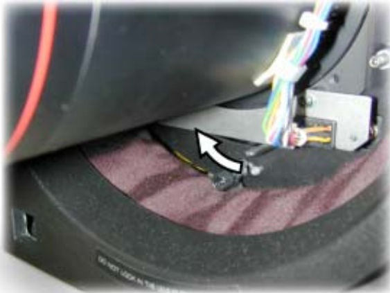
Image 1-2 Move the handle of the lens anchor system to the left
